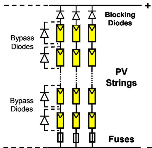
Fig. A11 - Protective devices in a PV generator
