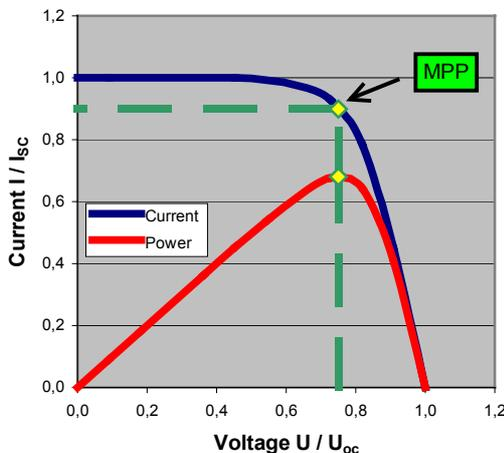
Fig. A4 - Module characteristics
