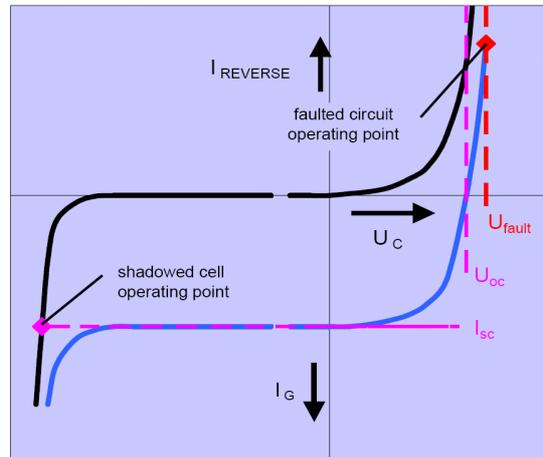
Fig.A9 - Shadowing and fault conditions
